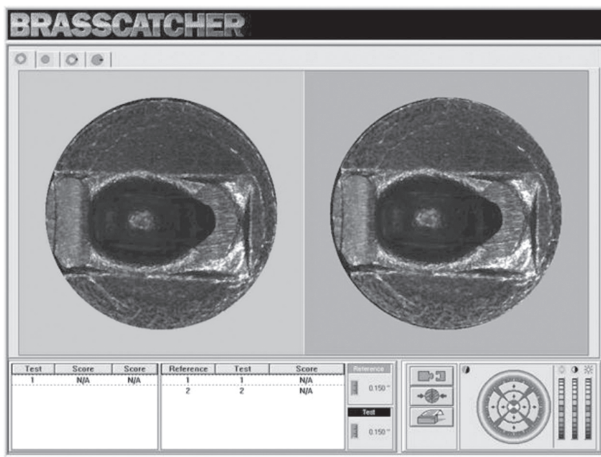
Figure 3: Side by side comparison of firing pin and breech face marks by the Brasscatcher module of IBIS
